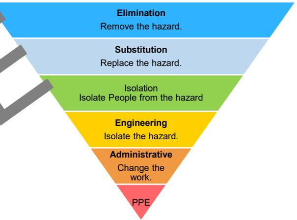
The pyramid shows five levels of controls from top to bottom: Elimination (Remove the hazard), Substitution (Replace the hazard), Isolation (Isolate People from the hazard), Engineering (Isolate the hazard), and Administrative (Change the work). PPE is shown as a separate level at the bottom.
